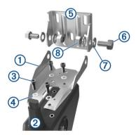
2 Attach the transducer mount bracket to the transom mount bracket (5) using the bolts (6), flat washers (7), and lock nuts (8).
