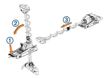
**NOTE:** The motor may automatically steer to 90° for stowing. The propeller stow side can be configured in the settings menu.
