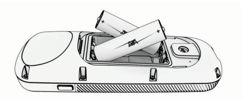
3 Replace the battery cover, and turn the D-ring clockwise.
